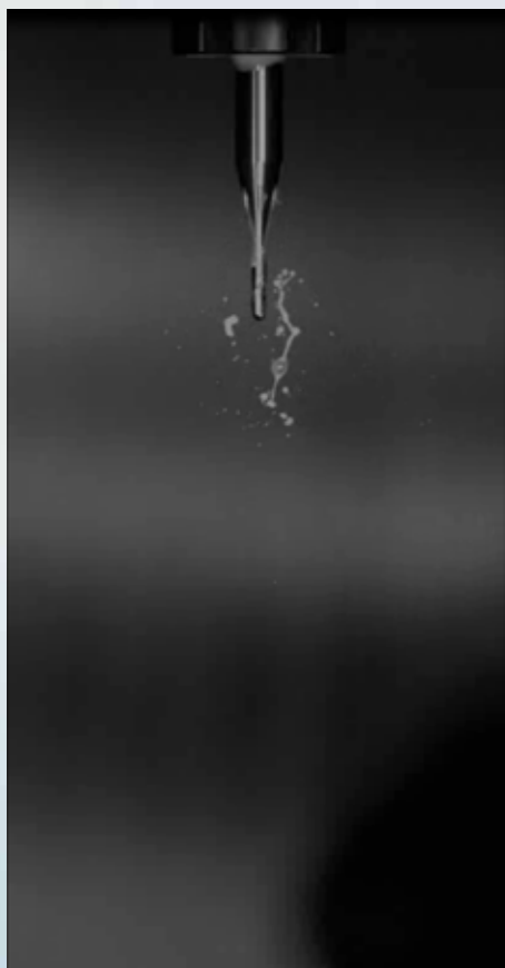
Switching on GuhroJet internal cooling
