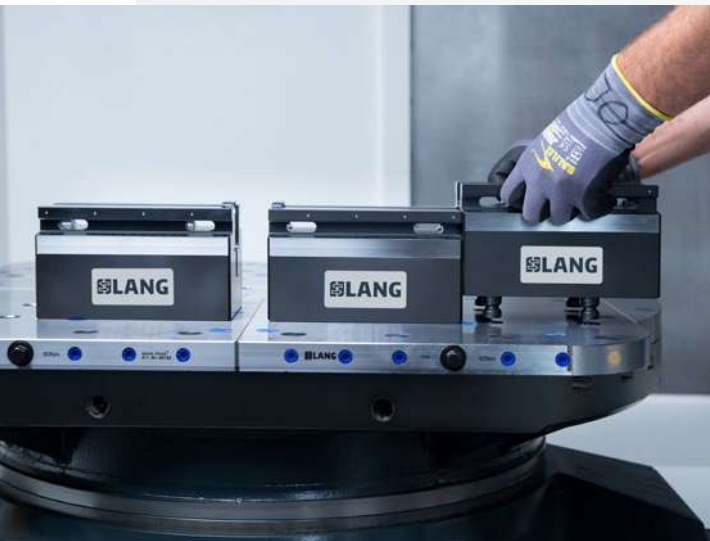
Adding further bases for an increased clamping range
