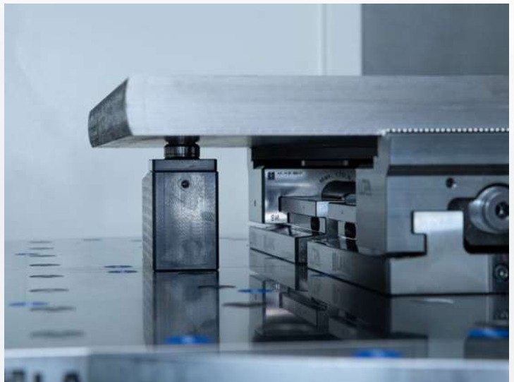
Low-vibration clamping using the Hydro-Sup screw jack
