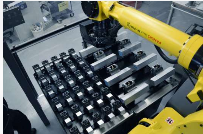
RoboTrex 96 with gripper exchange interface and different sizes of trolleys. Image: Waibel GmbH CNC-Teilefertigung
