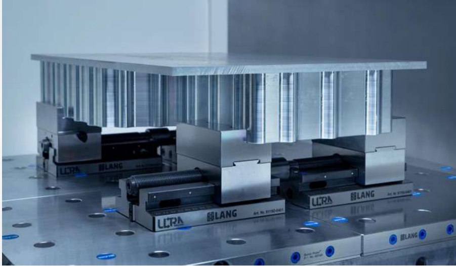
2nd OP / rear-face machining using contour jaws.
