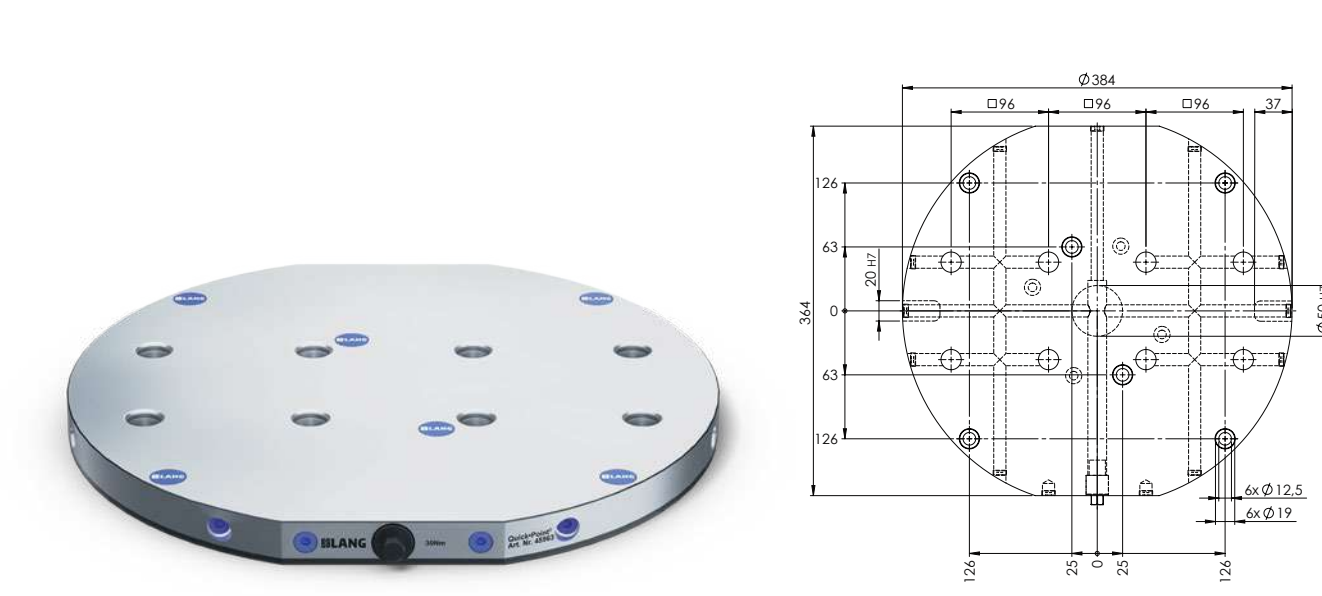
QUICK-POINT® 96, 2-FOLD GRID PLATE, ROUND Ø 384 × 27 MM, WITH MOUNTING BORES FOR 63 MM T-SLOT DISTANCE
