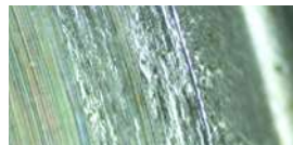
Bare metallic clamping nut after 15 clamping cycles
